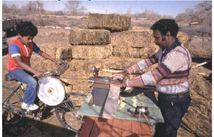
Operating a wood working lathe.
